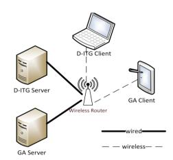
Fig. 3 Laboratory testbed
